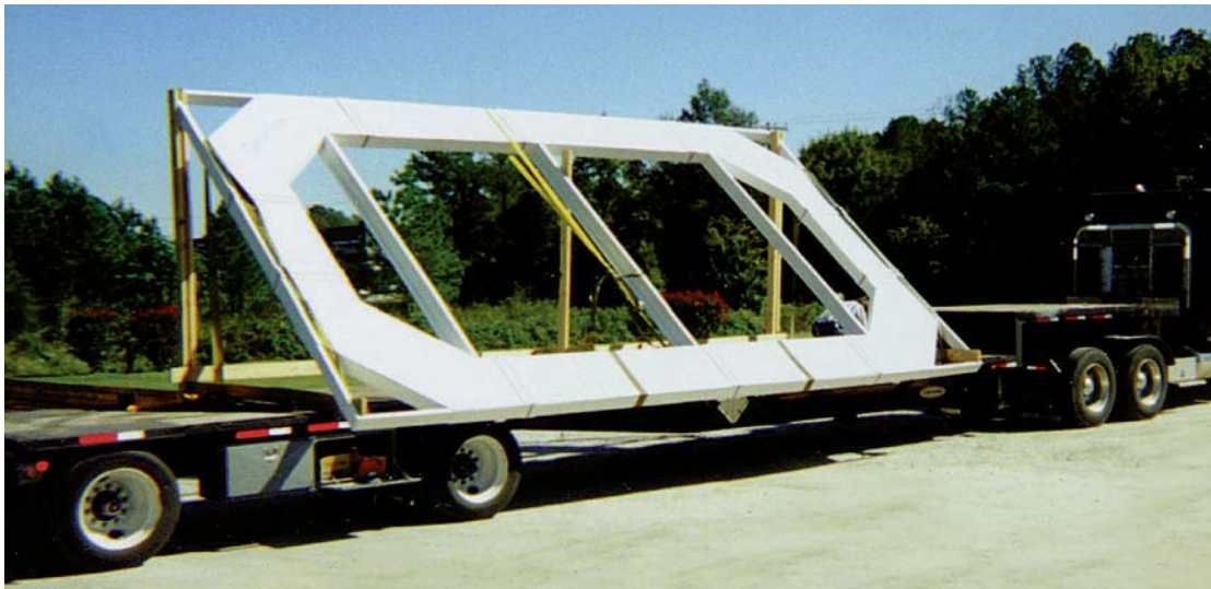
Wooden shipping crate for Reactor Pressure Vessel Seal
