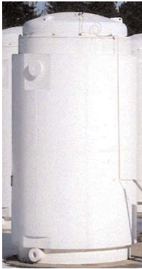
TN-32 Dry Storage Cask
